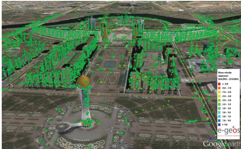
Figure 6 - 3D view of the PS mean velocity measurements obtained by PSP-IFSAR processing of COSMO-SkyMed images acquired from 2011 to 2014 over Astana
