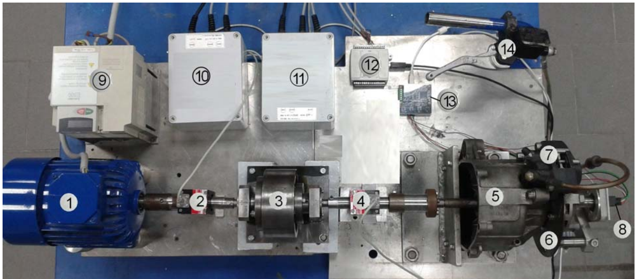
1-motor; 2 and 4- torsionmeter; 3-planetary transmission; 5-gearbox; 6-brake disk; 7-brake caliper; 8-encoder; 9-inverter; 10 and 11-amplifier; 12-NI data acquisition card; 13-Phidget data acquisition card; 14-brake lever.
